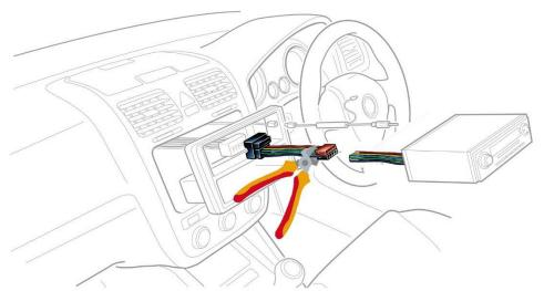
2. Once you have cut off the connectors you will need to join the loose wires of our Steering Wheel Control to the Chinese ISO accordingly.
